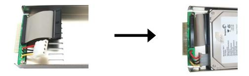
The 4 pin connection is the DC power cable for HDD, and the wider cable is the standard hard drive IDE type connection.
